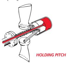
Pitch is decreased by allowing oil to flow out of the propeller and be returned to the engine sump. When the governor initiates this procedure, hydraulic pressure is decreased and the piston moves forward, moving the blades towards low pitch. The piston will continue to move forward until the opposing forces are again equal.
