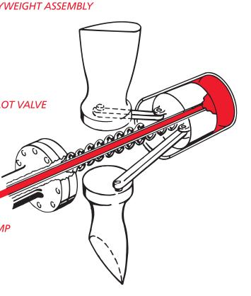
the position of the pilot valve. Depending on its position, the pilot valve will direct oil flow to the propeller, allow to flow back from the propeller, or assume a neutral position with no oil flow. As we saw earlier, these oil flow conditions correspond to increasing pitch, decreasing pitch or constant pitch of the propeller blades.
