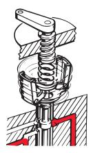
As engine RPM increases, the tops of the weights are thrown outward by centrifugal force. The lower legs then pivot up, raising the pilot valve against the force of the speeder spring, so there is no oil flow to or from the propeller.
