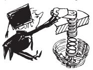
Thus, with the cockpit control, the aircraft pilot can shift the range of governor operation from high RPM to low RPM or any area in between.
