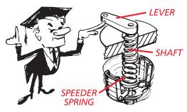
For example, when the cockpit control moved forward, the governor control shaft is screwed down, increasing compression on the spring. This means that the flyweights must spin faster to raise the pilot valve, which results in a higher RPM setting.
