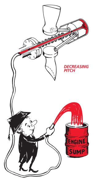
Although they aren't shown in our illustrations, mechanical stops are installed in the propeller to limit travel in both the high and low pitch directions.
