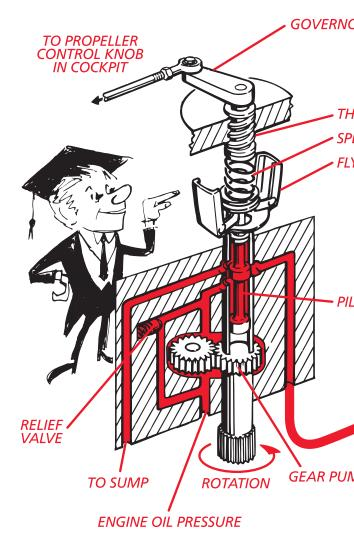
A look at the total system will help to explain this. Besides the propeller, the other major component of the system is the governor. The governor mounts on, and is geared to, the engine. This drives the governor gear pump and flyweight assembly. The gear pump boosts engine oil pressure to provide quick and positive response by the propeller. The rotational speed of the flyweight assembly varies directly with engine speed and controls
