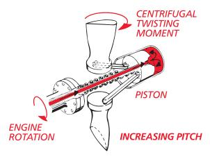
In the propeller, oil pressure acting on the piston produces a force that is opposed by the natural centrifugal twisting moment of the blades and a spring. To increase the pitch or blade angle, we direct high pressure oil to the propeller. This moves the piston back. Motion of the piston is transmitted to the blades through the actuating link and pins, moving the blades toward high pitch.
